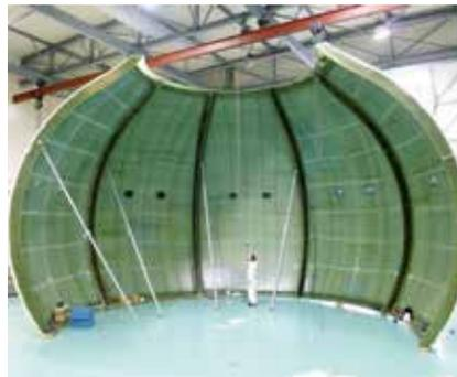
// Five gilded domes of the Russian Orthodox Cathedral in Paris, France. The domes were manufactured off-site and it took 15 minutes to put the largest dome, spanning 12 metres in diameter, in place by crane.
